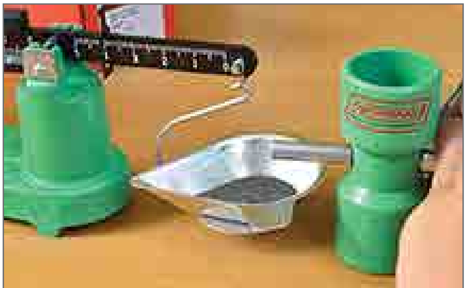
Example 14: Fill the pan with the Trickler until beam is in balance
